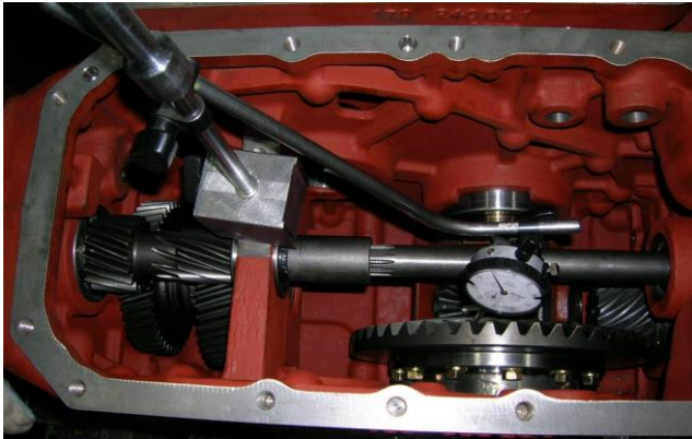
Adjust the shimming to backlash
